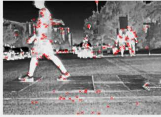
Figure 11. Corner Detection using FAST algorithm
