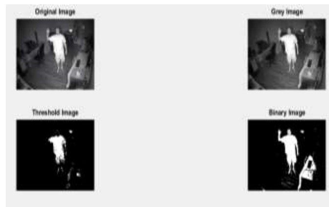
Figure 7. Original output of night vision camera image (Top left), Grey scale image (top right), Threshold binary image (bottom left), simple binary (bottom right).
