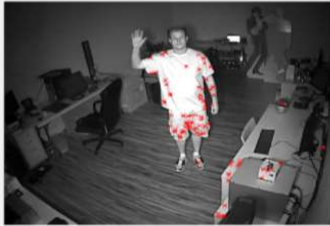
Figure 8. Corner Detection using FAST algorithm
