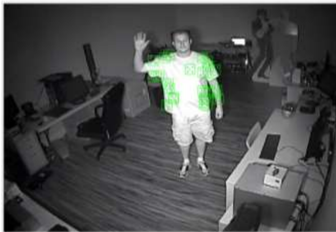
Figure 9. Feature Extraction using HOG Algorithm.
